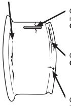
Circumferential cracks in middle of rim.
